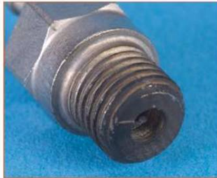
A blown plug is often the result of a foreign particle getting into the combustion chamber. As long as the coil remains intact, the engine should run until the motor is turned off for that flight.
