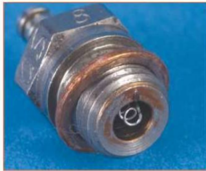
Example of a plug pulled from a well-tuned engine.
