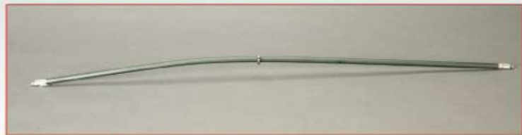
This torque tube is bent and cannot be used. Do not try and bend it back.
