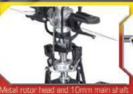
Metal rotor head and 10mm main shaft
