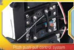
Pitch push-pull control system
