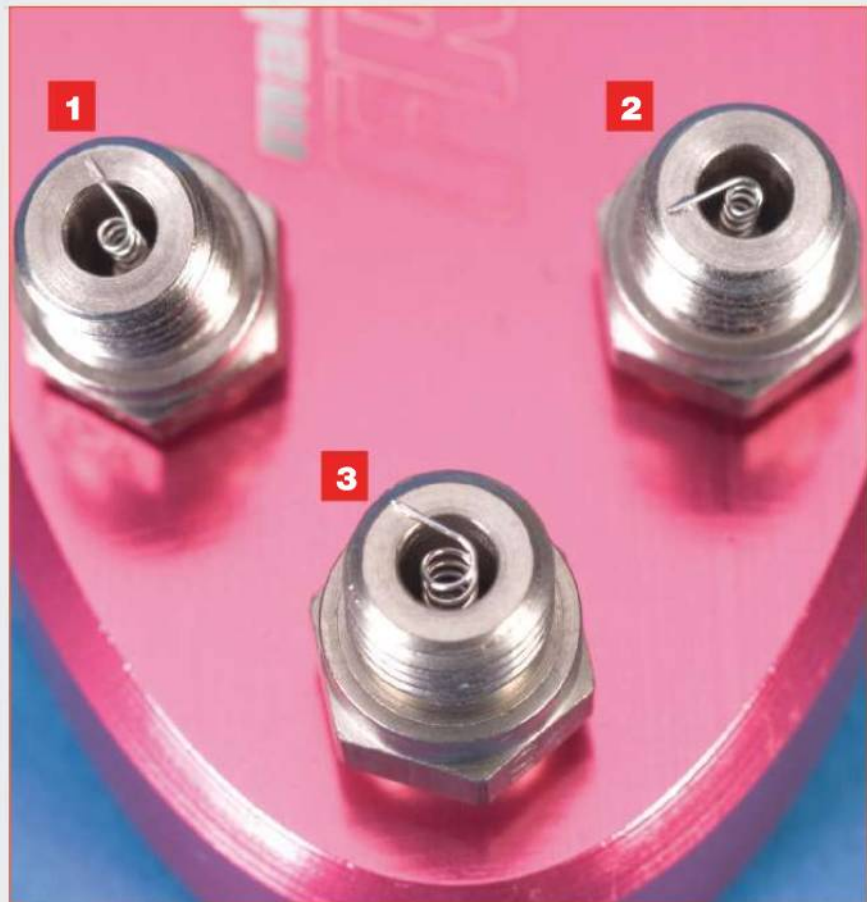
Here is an example of the coil thicknesses of some hot, medium, and cold plugs. Hot is on the left and cold is on the right. Notice the thinner filament on the hot plug.
