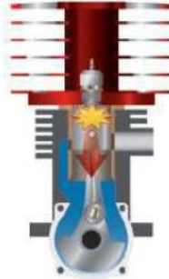
The coil glows red hot when given a little electricity.
